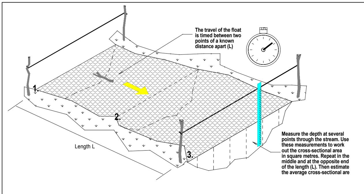
Figure 7-6 The float method of flow measurement
