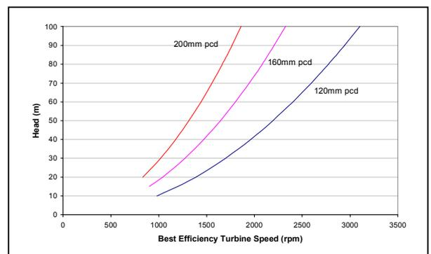
Figure 8-7 Graph showing the operating range of three Pelton runner diameters
