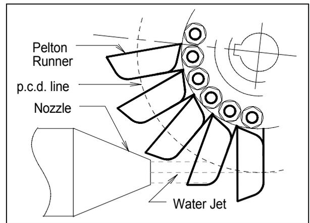
Figure 8-6 The Nozzle directs the water jet on to the p.c.d. line of the turbine runner
