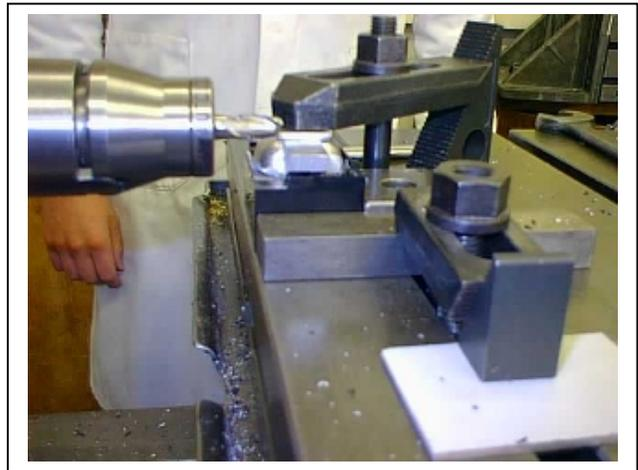
Figure 3 Machining reference surface on bucket
