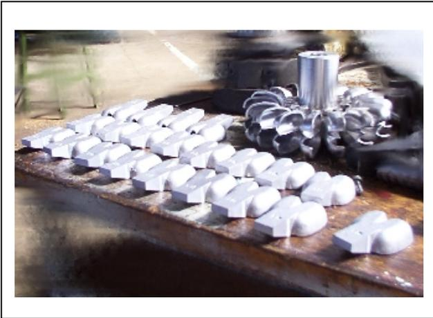
This section provides guidance for the manufacture and assembly of small Pelton turbine runners from individual bucket castings.
